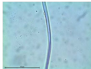
Figure 2: Fibres from a silk fabric dyed in the Abegg-Stiftung without particles on the surface.
