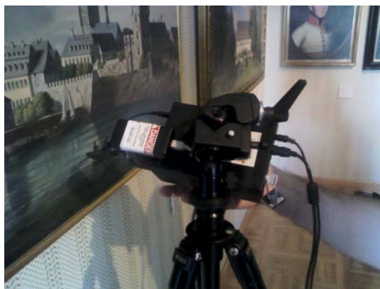
Figure 1. Raman experiment of “Vukovar landscapes” painting in Eltz Manor, Vukovar, Croatia.
