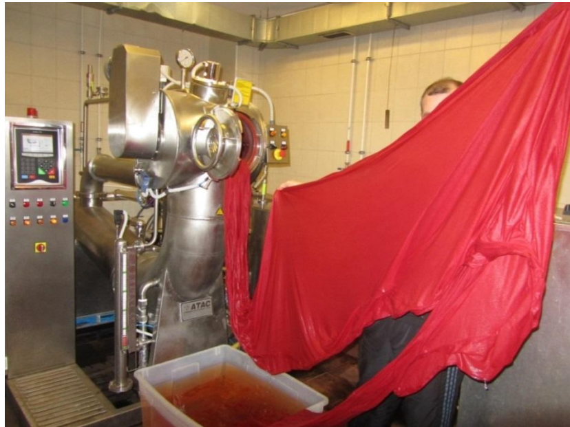
Fig. 1: Modified and developed dyeing machine for natural dyes.
